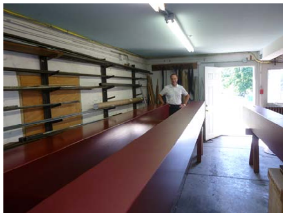
Here I am standing between two “open woods,” what will be among the largest pipes in the organ.
